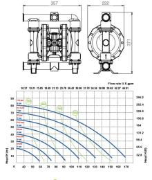
• Air supply pressure • Air consumption Nit/min [SCFM] The curves and performance values refer to pumps with submerged suction and free delivery outlet, with water at 20°C. These data may vary according to the construction materials and hydraulic conditions.
