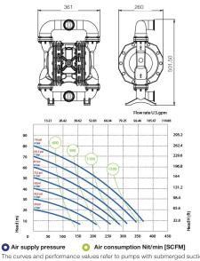
The curves and performance values refer to pumps with submerged suction and free delivery outlet, with water at 20°C. These data may vary according to the construction materials and hydraulic conditions.
