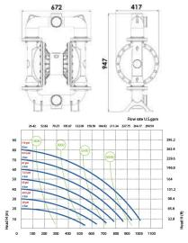
O Air supply pressure Air consumption Nit/min [SCFM] The curves and performance values refer to pumps with submerged suction and free delivery outlet, with water at 20°C. These data may vary according to the construction materials and hydraulic conditions.
