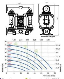
O Air supply pressure O Air consumption Nit/min [SCFM] The curves and performance values refer to pumps with submerged suction and free delivery outlet, with water at 20°C. These data may vary according to the construction materials and hydraulic conditions.
