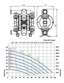
• Air supply pressure • Air consumption Nit/min [SCFM] The curves and performance values refer to pumps with submerged suction and free delivery outlet, with water at 20°C. These data may vary according to the construction materials and hydraulic conditions.
